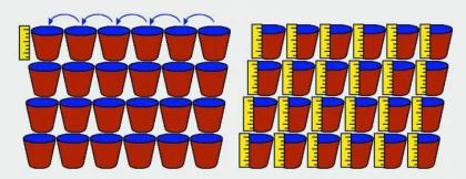
CCD sensors have one readout in corner, while CMOS sensors have readout at each pixel.
