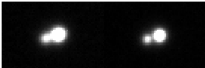
Double star image without AO (left) and with AO (right). Both images are 15 minute exposures, enlarged 300%
